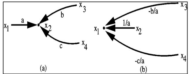
Fig. 2: Signal flow graph of (a) Eq. (3) and (b) Eq. (4).
