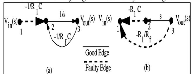
Fig. 5: Original and inverted SFGs for integrator.
