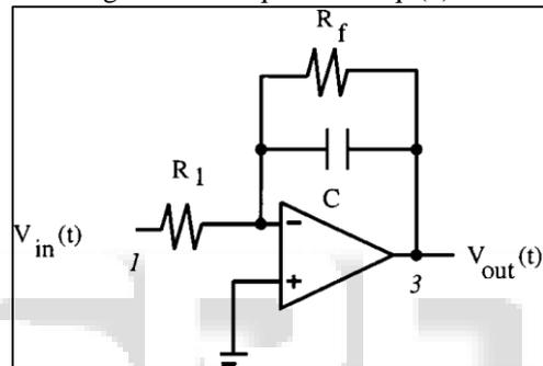
Fig. 3: Real Integrator circuit.
