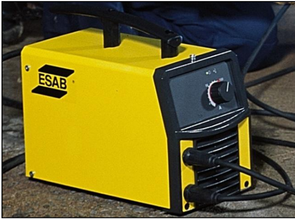
Fig. 2.1: ESAB make welding machine
