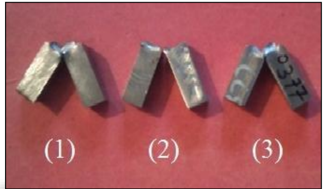
Fig. 3.1: Impact test specimens after fracture
