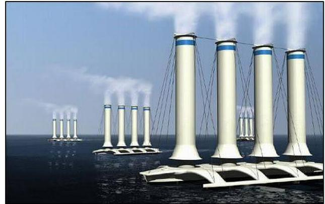
Fig. 1: Proposed geo engineering spray vessel
