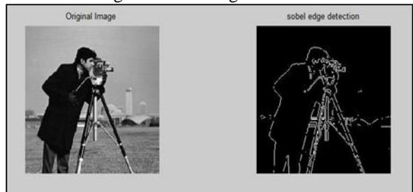
Fig. 5: Example of Sobel edge detection technique.
