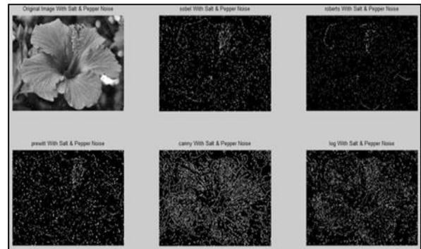
Fig. 16: Edge detection technique with Salt & Pepper Noise.
