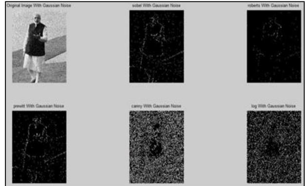
Fig. 11: Edge detection technique with Gaussian Noise.
