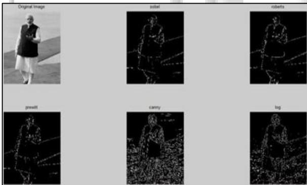
Fig. 9: Edge detection technique on original Image.
