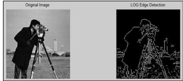
Fig. 8: Example of LOG edge detection technique.
