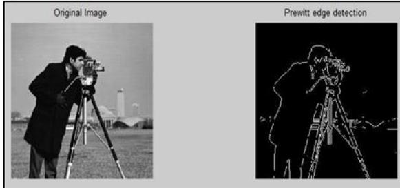
Fig. 6: Example of Prewitt edge detection technique.
