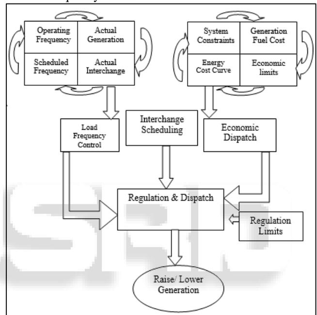
Fig. 1: Automatic Generation control
