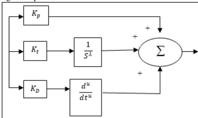
Fig. 2: FOPID controller structure
