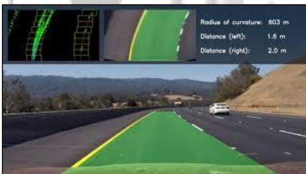
So these is a major problem in Self-Driving Car, to avoid it we can use 360 degree HD camera along with ultrasonic sensor or lidar sensor. Camera will be used in Object detection and Road Detection. Here is a Game Changer Lidar sensor give give thermal outline uptila a particular range its just like small 3D graph. This will not only help in Road Detection but also whats around the Car.
