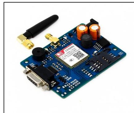
Fig. 6: GSM Module
