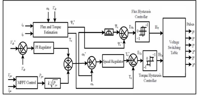
Fig. 3: DTC scheme of the proposed system
