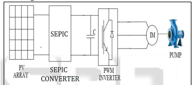
Fig. 1: Configuration of proposed system
