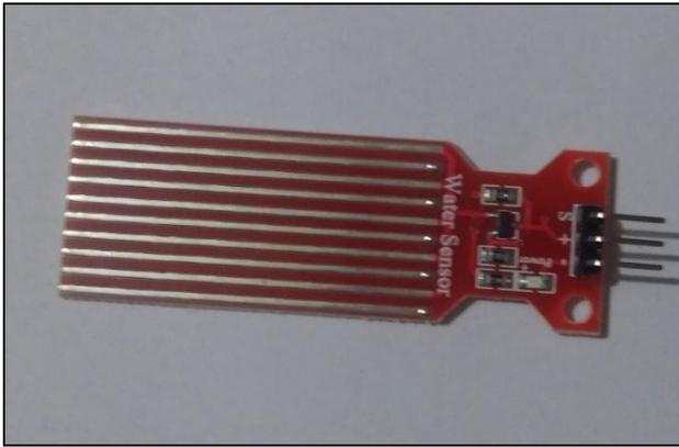
Fig. 3: water level sensor
