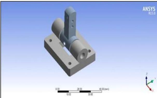
Fig. 3.5: Modelled Steering Seat Base and Arm Assembly for CF PLA
