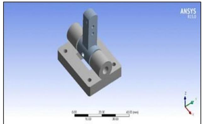
Fig. 3.1: Modelled Steering Seat Base and Arm Assembly for PLA
