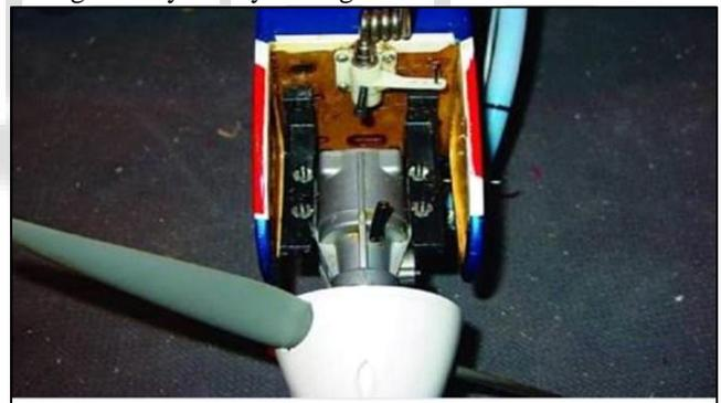
Fig. 2: RC Aircraft Front Wheel Steering Part
