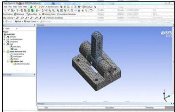
Fig. 3.6: Meshing of Steering Seat Base and Arm
