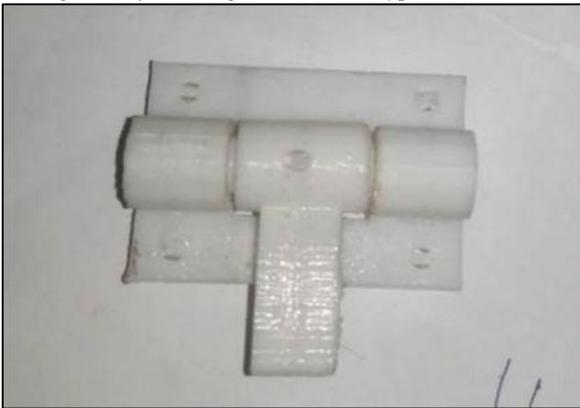
Fig. 4.3: Fabricated seat base and arm by using PLA
