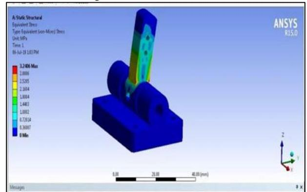
Fig. 3.9: Equivalent Stress
