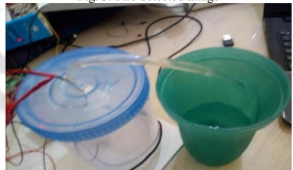
Fig. 6: Fire extinguish (using submersible motor and Water sprinklers)
