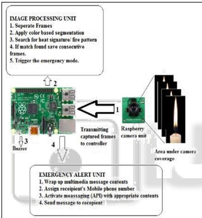
Fig. 2: working process of raspberry
