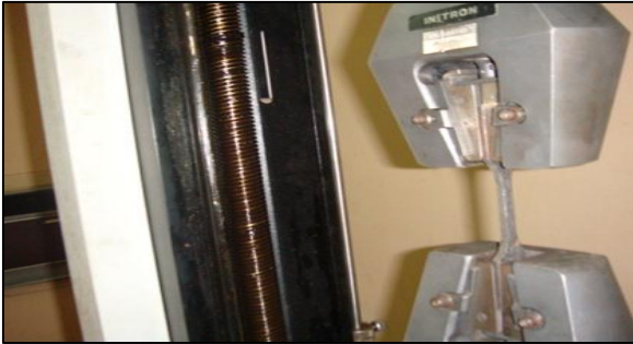
Fig. 8: Instron 1195 machine for tensile test
