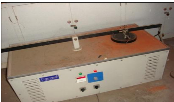
Fig. 6: Pin on disc machine for abrasive wear testing.
