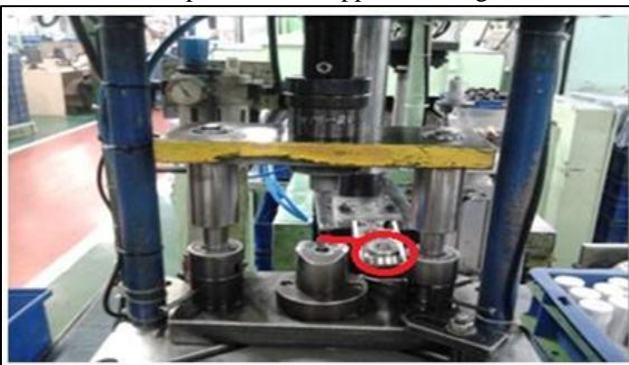
Fig. 10. improved bearing squeezing Issue 5: Work station: Bearing squeezing and oil apply
