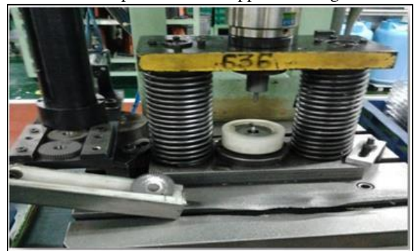
Fig. 8: Improved driven apparatus squeezing
