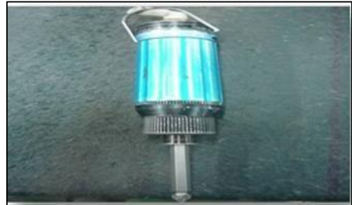
Fig. 11: Pneumatic Air Gun for burden fixing
