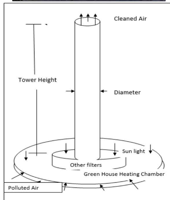
Fig. 2: The proposed Roosegaarde type tower and some functional details
