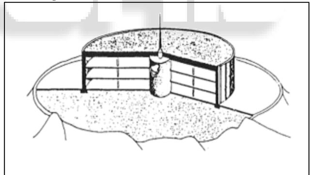
Fig. 8: Three-level concrete lunar base proposed by Lin et al. (1989)
