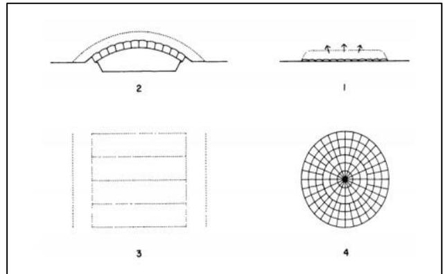
Fig. 1: Base concept, low arch shield with a pneumatic support structure (Land 1985, courtesy of NASA). (1) Deflated structure flat structure flat on the ground. (2) Structure inflated, raising the regolith. (3) Plan showing the concept applied in sections for a concept applied in sections for a continuous low arch shield. (4) Plan showing concept applied in a low domed shield
