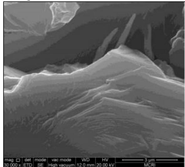
Fig. 2: SEM micrograph of tensile fracture surface of 0.5 wt % CNTs/ Ti-6Al-4V composites
