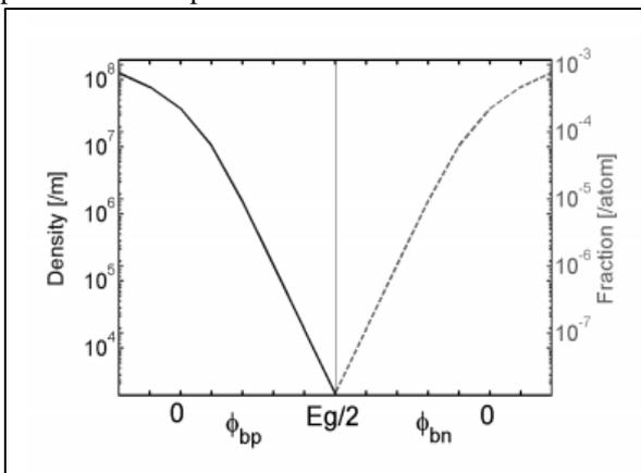
Fig. 5: Electron density and the hole density in the center
