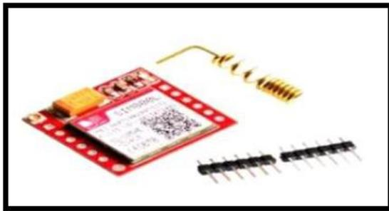
Fig. 5: GSM modem
