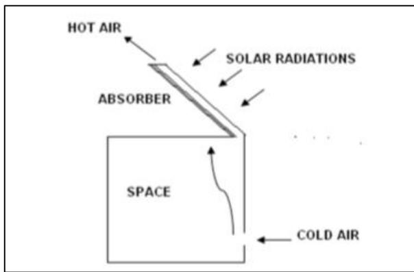
Fig. 1: Concept of Solar Chimney
