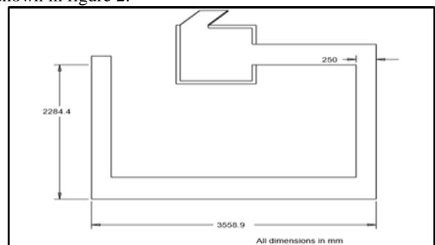
Fig. 1: Schematic of inclined solar chimney with Geothermal Heat Exchange Design
