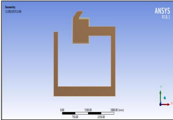
Fig. 2: Imported CAD model of inclined solar chimney with Geothermal Heat Exchange
