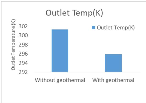
Fig. 7: Outlet Temperature comparison
