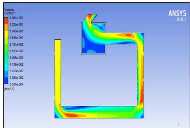
Fig. 6: Velocity plot of geothermal mechanism
