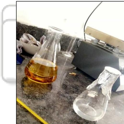
Fig. 2: Vegetable Oil and Potassium Methoxide
