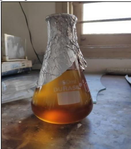
Fig. 3: Solution of Vegetable oil and Potassium Methoxide
