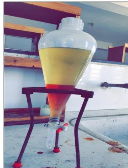
Figure 4:- Layer formation of biodiesel and Glycerol in separating funnel.
