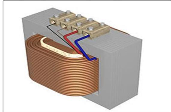
Basic diagram of a Transformer
