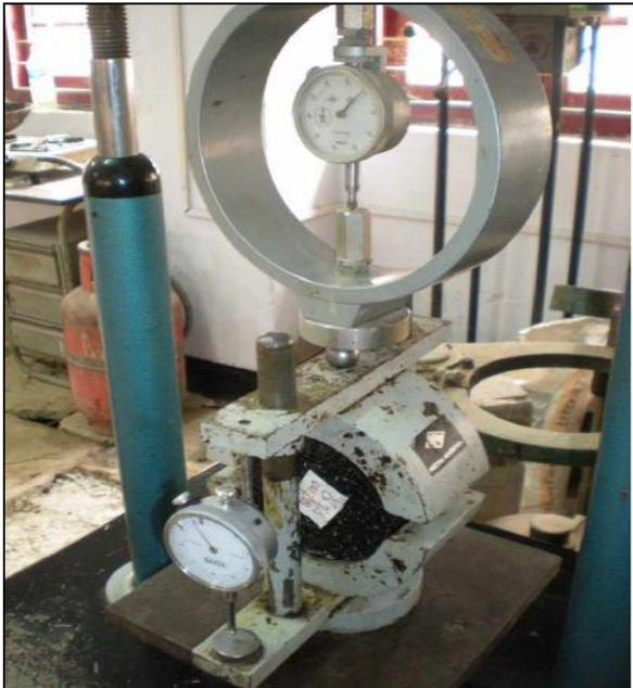
Fig. 2: Marshall Test in Progress
