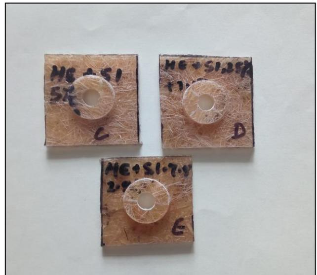
Fig. 6: Shear Test specimen
