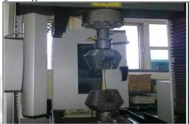
Fig. 1: Universal testing machine
