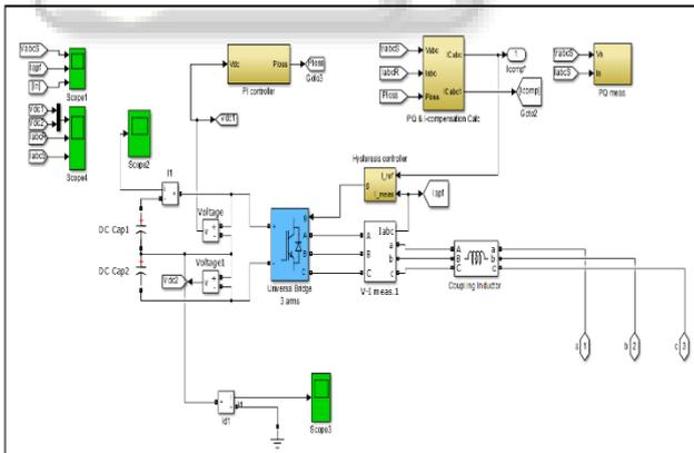
Fig. 5: MATLAB simulation model of shunt controller
