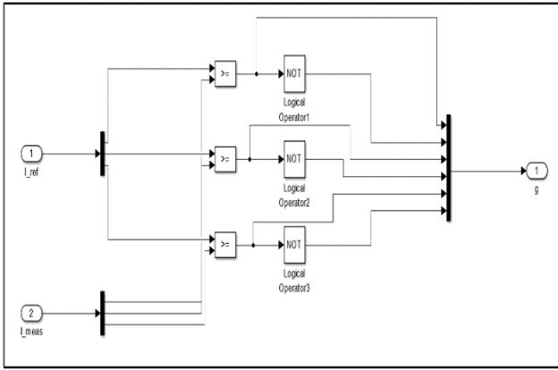
Fig. 8: Hysteresis based Ireference and Imean current comparison subsystem model
