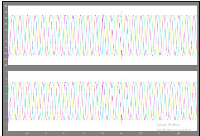
Fig. 11: Receiving end three phase voltage and current of transmission line without voltage swell and sag
