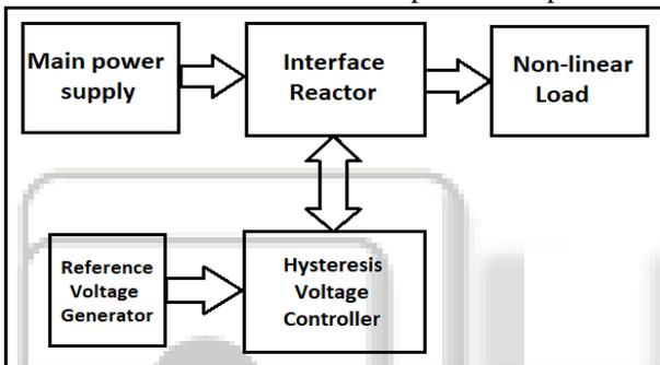
Fig. 4: Block diagram of proposed series active power controller
