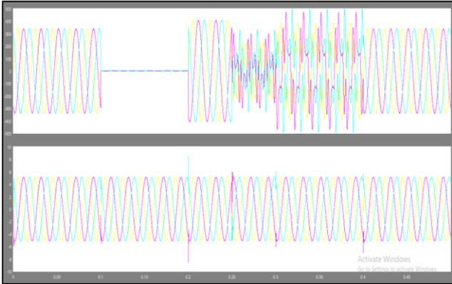
Fig. 12: Sending end three phase voltage and current of transmission line with harmonics and interruption condition
