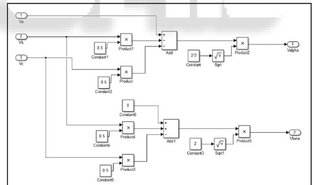
Fig. 6: Clarke transformation for Valpha and V beta Calibration
