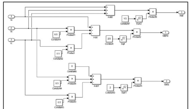
Fig. 7: Clarke transformation for Ialpha and I beta Calibration
