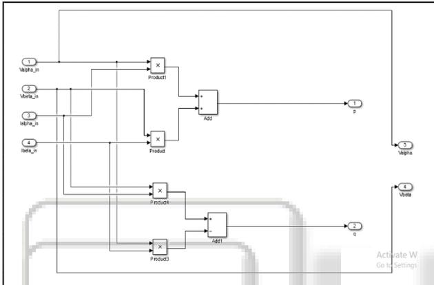
Fig. 9: P and Q components calibration subsystem model
