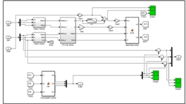
Fig. 5: PQ components calibration subsystem model
