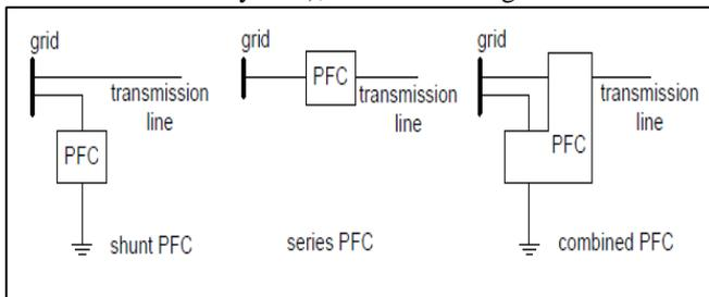
Fig. 1: Simplified diagram of shunt, series and combined devices
