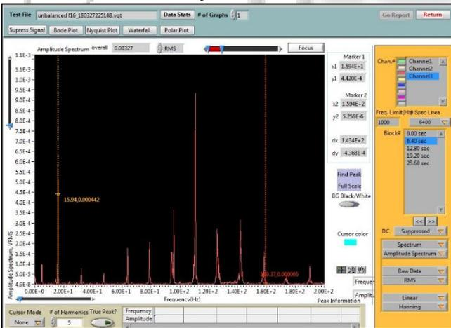
Fig. 3.4: Vibration spectrum at NDE of unbalanced rotor at rotor speed of 16 Hz
