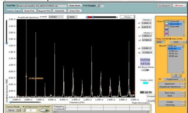
Fig. 3.1: Vibration spectrum at DE of balanced rotor at rotor speed of 16 Hz
