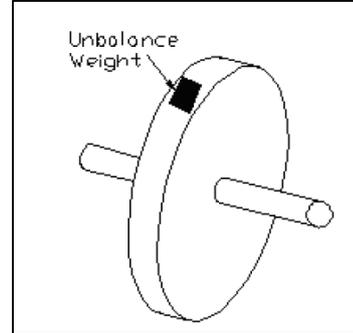
Fig. 5.1: Thin rotor with single plane unbalance
