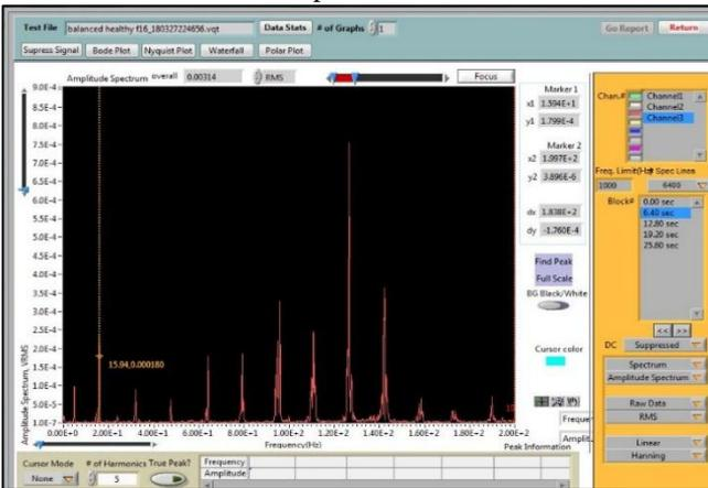
Fig. 3.3: Vibration spectrum at NDE of balanced rotor at rotor speed of 16 Hz
