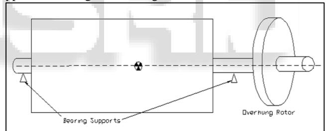
Fig. 5.3: A typical configuration of an overhung rotor
