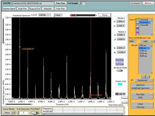
Fig. 3.2: Vibration spectrum at DE of unbalanced rotor at rotor speed of 16 Hz
