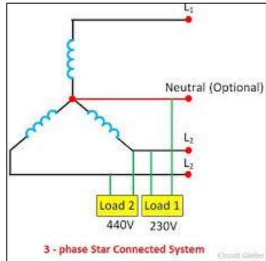
Fig. 2: 3- Phase Connection System
