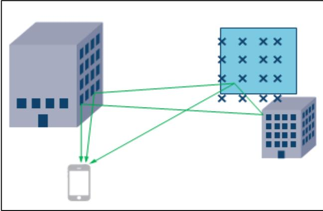
Fig. 5: Multipath environment between antenna array and user.
