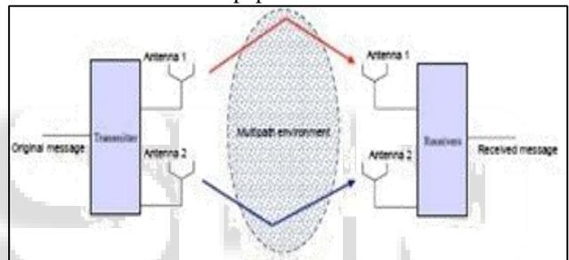
Fig. 1: Point-to-point MIMO links.
