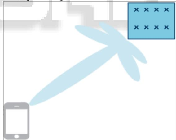
Fig. 4: Traditional beamforming.
