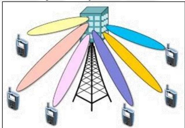
Fig. 2: Multiuser MIMO (MU-MIMO) antenna system.
