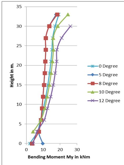
FOR COLUMN 1:- Result of the forces in 10 degree building frame with lateral ties.
