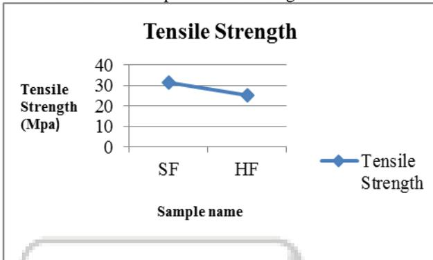
Fig. 7: Tensile properties of sisal and hemp fiber
