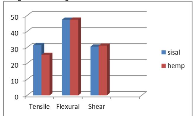
Fig. 9: Comparison of mechanical properties of sisal and hemp fiber
