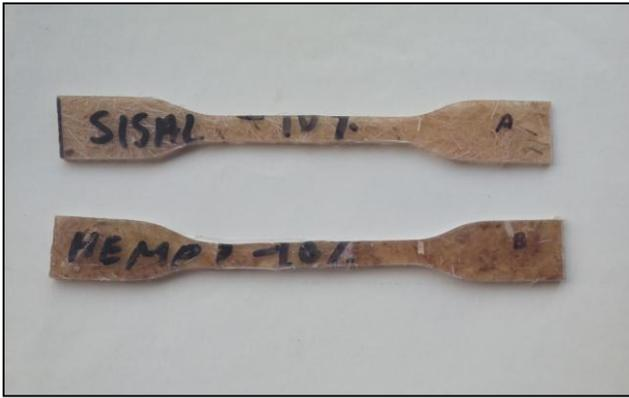
Fig. 2: Tensile test specimen
