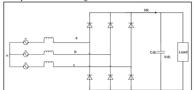
Fig. 3. Three-Phase Full Diode Bridge Rectifier
