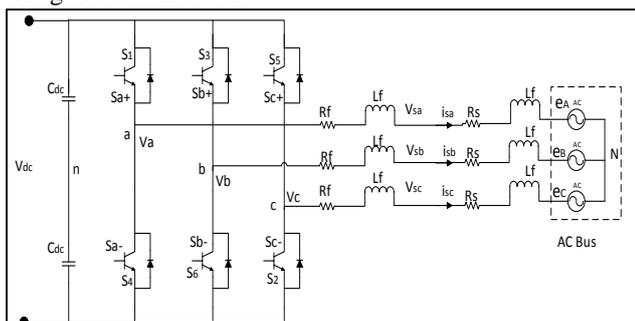
Fig. 5: 3-Phase DC/AC Inverter
