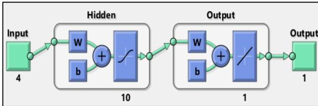
Fig. 2: Architecture of Artificial Neural Network Based MPPT for WECS
