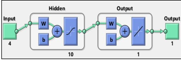
Fig. 1: Architecture of Artificial Neural Network Based MPPT for PV system
