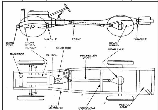
Fig. 1: Layout of Chassis [1]
