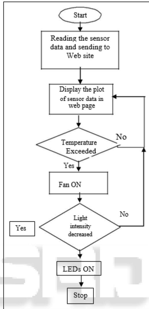
Fig. 6: Flow Diagram
