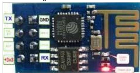
Fig. 2: ESP8266 Pin Details
