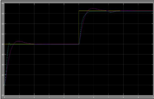
Fig. 18: comparison of response of PID (Purple) and FLC (Blue) with respect to reference speed (Yellow)
