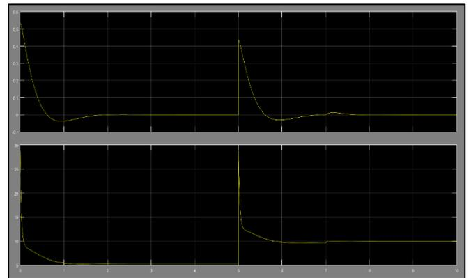
Fig. 5: Upper graph for speed error in pu while lower graph for corresponding armature voltage using PID controller as APS
