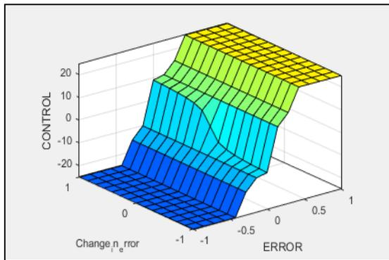
Fig. 14: Fuzzy logic controller controlling surface in MATLAB simulink
