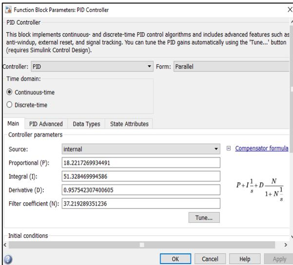
Fig. 3: PID controller gain values after successful tuning in MATLAB simulink
