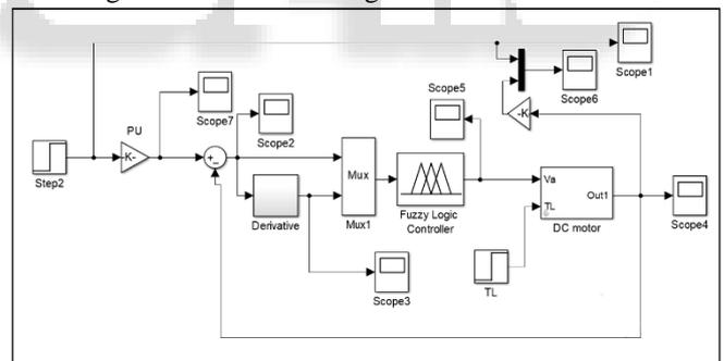
Fig. 6. Proposed matlab simulation model for DC motor power system
