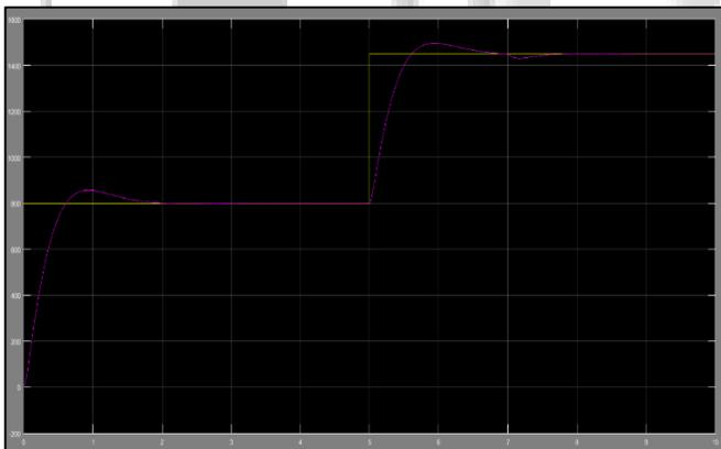
Fig. 4: Reference speed vs PID controller controlled speed graph in MATLAB simulink scope
