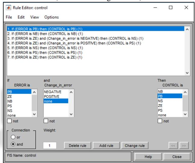
Fig. 12: Fuzzy rule base designing window in MATLAB simulink
