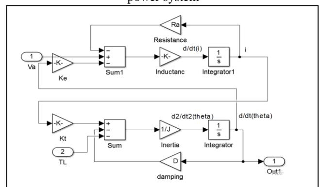
Fig. 7: DC motor modeling in MATLAB simulink
