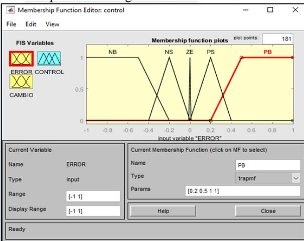
Fig. 9: Fuzzy membership function designing for speed ERROR signal
