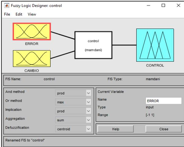
Fig. 8: Fuzzy logic controller design tool in MATLAB simulink
