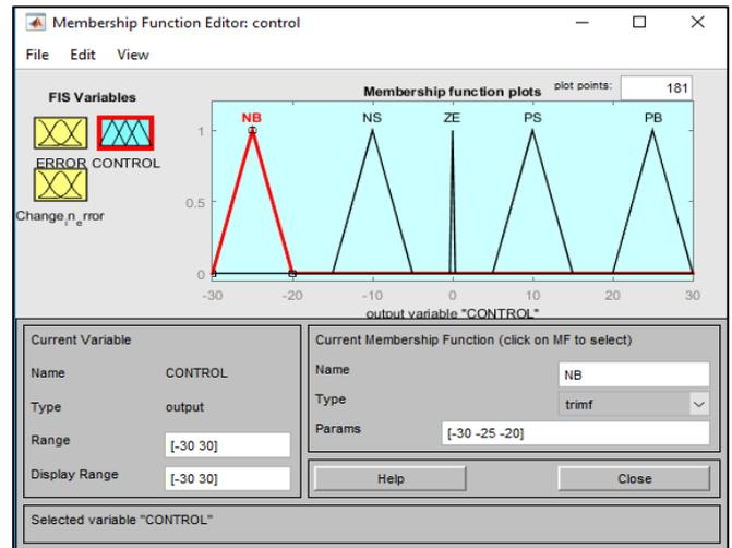
Fig. 11: Fuzzy membership function for control output (Armature voltage control)
