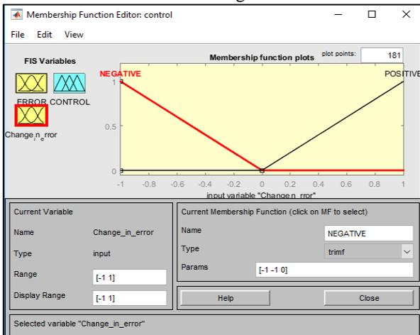
Fig. 10: Fuzzy membership function for speed change in error signal
