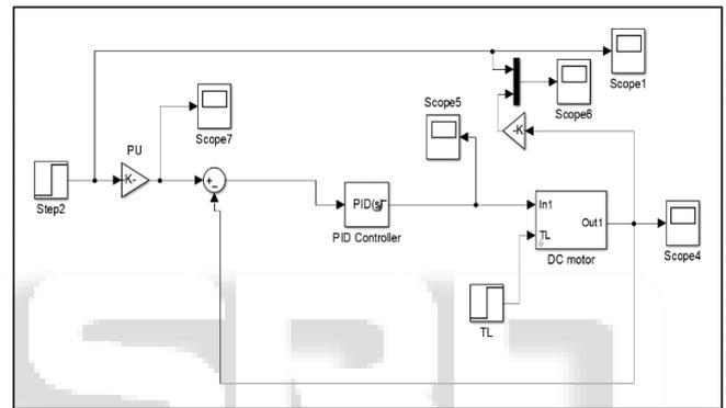
Fig. 1: MATLAB simulink model for APS for DC motor using PID controller
