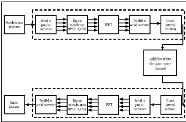
Fig. 2: Working Model of OFDM for Simulation
