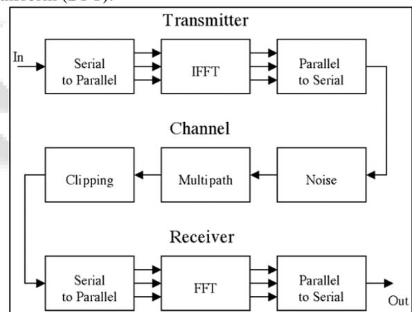
Fig. 1: Block Diagram of OFDM Model
