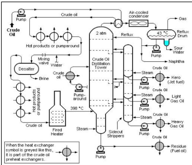
Fig. 4: Crude oil atmospheric distillation process [42]
