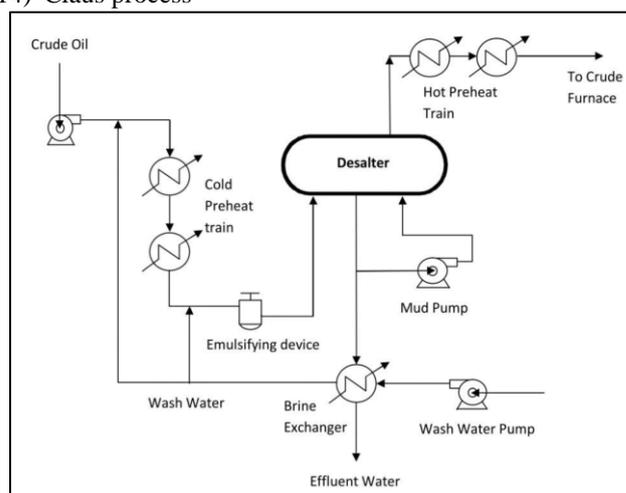
Fig. 3: Crude oil desalting process [41]
