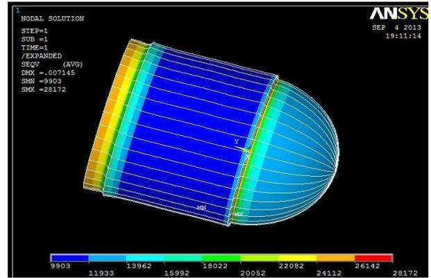
Fig. 5.2: Maximum Displacement in cylinder = 0.007145mm
