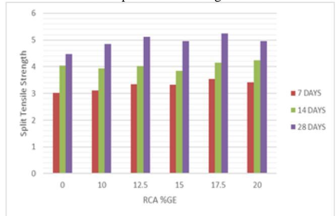
Fig. 4: Split Tensile Strength results
