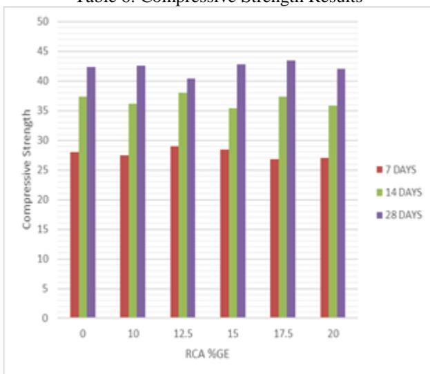
Fig. 3: Compressive Strength results
