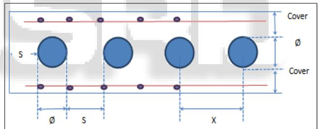
Fig. 3.2: Typical cross section of slab with top and bottom reinforcement
