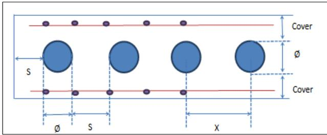
Fig. 2.1: Typical cross section of bubble deck slab used in current study
