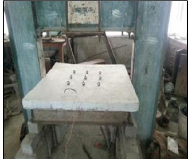
Fig. 3.1: Arrangement of Nine-point Load at the centre of the slab
