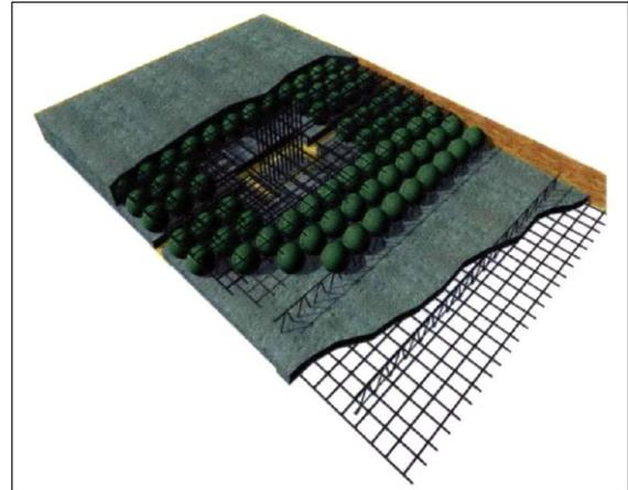
Fig. 1.1: Cut through section of Bubble Deck
