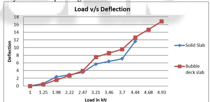
Fig. 5.1: Load deflection curve of solid and bubble deck slab.
