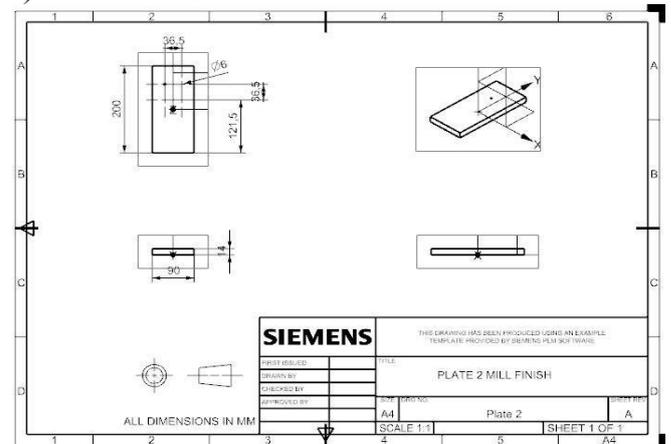
Fig. 9: Drafting of Vertical Plate
