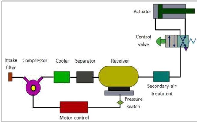
Fig. 6: Basic Pneumatic System
