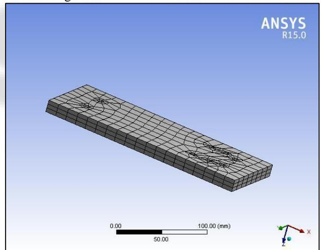
Fig. 15: Meshing of Horizontal Plate
