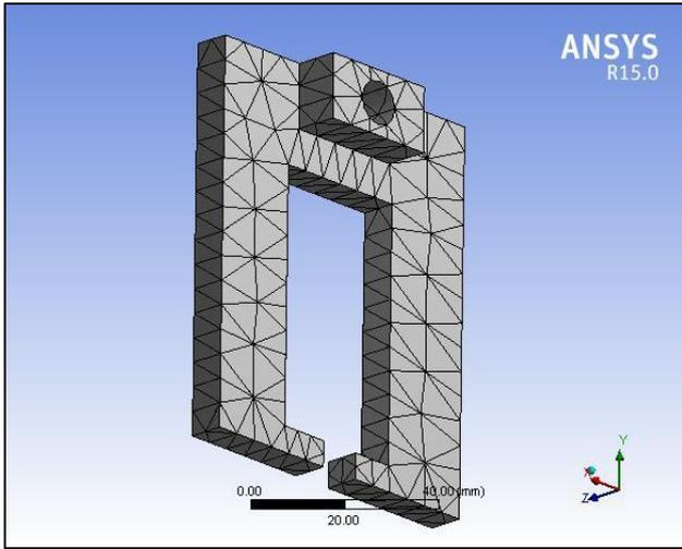
Fig. 11: Meshing of C-Plate
