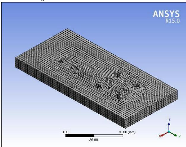
Fig. 17: Meshing of Vertical Plate
