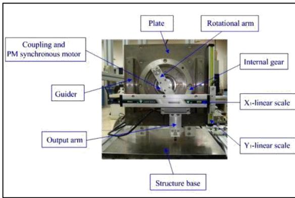
Fig. 4: Experimental Setup of Magnetic PPM
