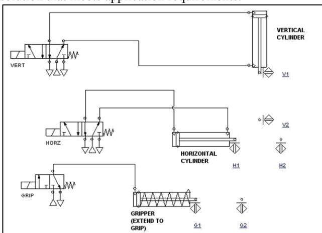
Fig. 5: Pneumatic Pick & Place System
