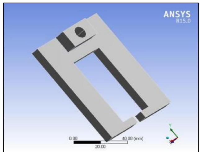
Fig. 10: CAD Model of C-Plate
