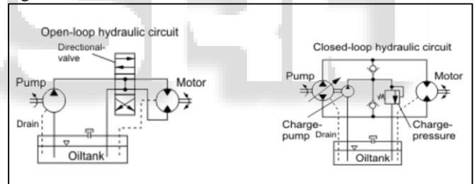
Fig. 2: Schematic of Hydraulic Pick and Place
