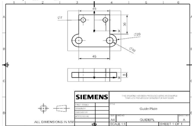
Fig. 8: Drafting of Guide Plate
