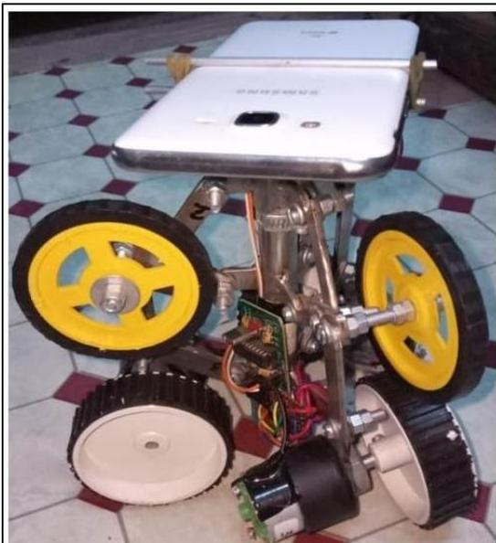
GSM Pipe Inspection Robot
