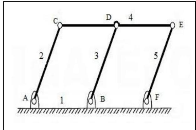
Fig. 1: Simple Parallelogram Mechanism
