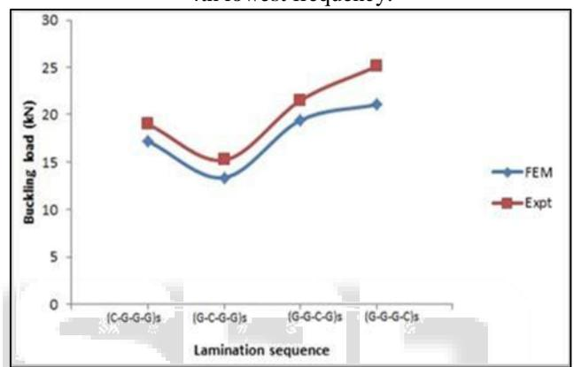
Fig. 6: Variation of buckling load with lamination sequence of CFRP plates in CFCF boundary condition with 25% carbon fibre.
