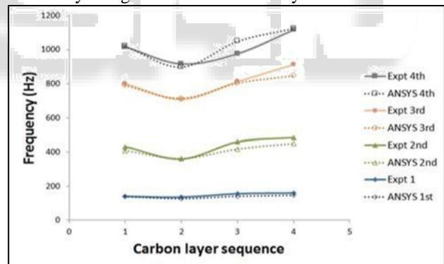
Fig. 1: Variation in natural frequency with the stacking sequence of carbon fibre in carbon/glass hybrid plates with 25 % carbon fibre
