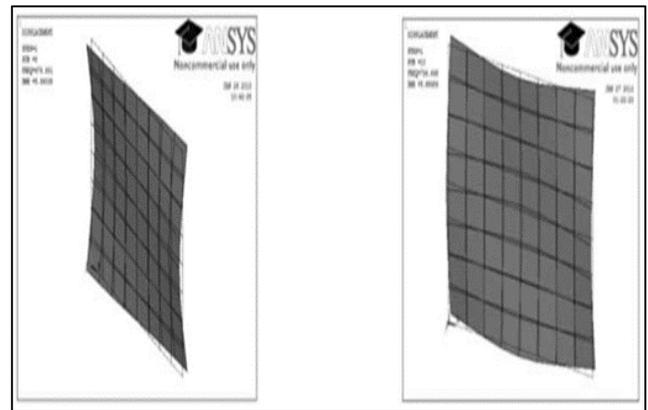
Fig. 5: Mode shapes for first four modes for 8 layered CFRP plate for FFFF boundary condition: (a) 1st lowest frequency, (b) 2nd lowest frequency, (c) 3rd lowest frequency and (d) 4th lowest frequency.
