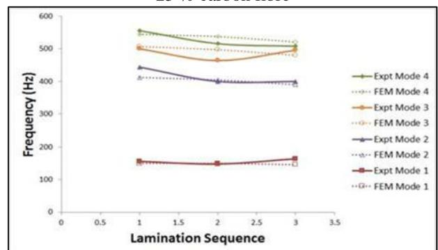
Fig. 2: Variation in natural frequency with the stacking sequence of carbon fibre in carbon/glass hybrid plates with 50 % carbon fiber
