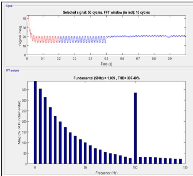
Fig. 4.7: Fast Fourier Transform and Total Harmonic Distortion of the input signal
