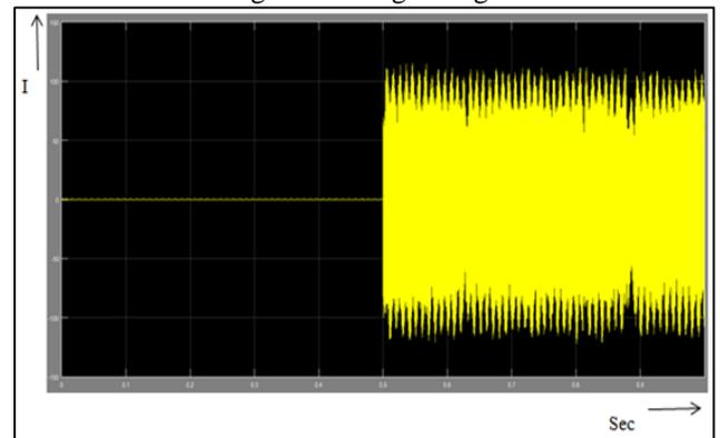
Fig. 4.4: Noise in input current
