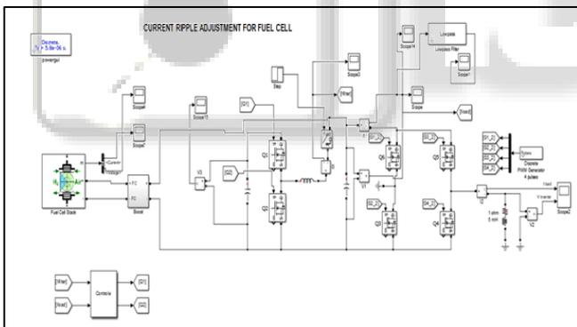
Fig. 3.1: Simulink model of current ripple adjustment for fuel cell
