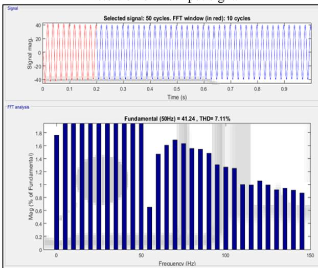
Fig. 4.8: Fast Fourier Transform and Total Harmonic Distortion of the output signal
