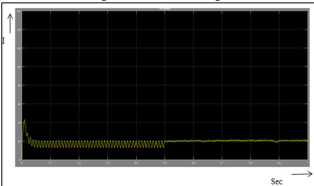
Fig. 4.2: Fuel cell current
