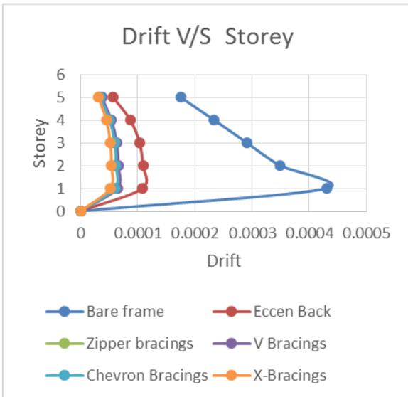
Fig. 5: Storey v/s Drift Plot for 5 storey structure in x direction (zone-2)
