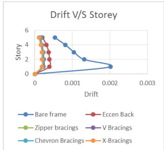
Fig. 8: Storey v/s Drift Plot for 5 storey structure in Y direction (zone-5)
