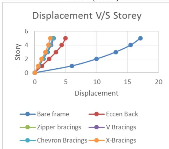
Fig. 4: Storey v/s Displacement Plot for 5 storey structure in Y direction (zone-5)
