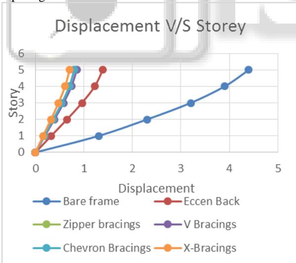
Fig. 1: Storey v/s Displacement Plot for 5 storey structure in x direction (zone-2)
