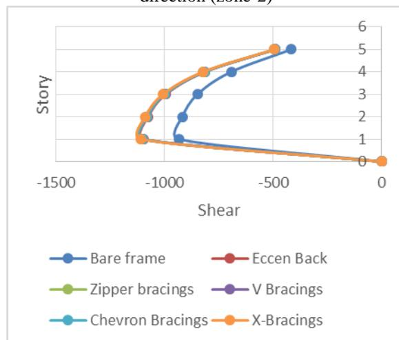
Fig. 10: Storey v/s storey shear Plot for 5 storey structure in X direction (zone-5)
