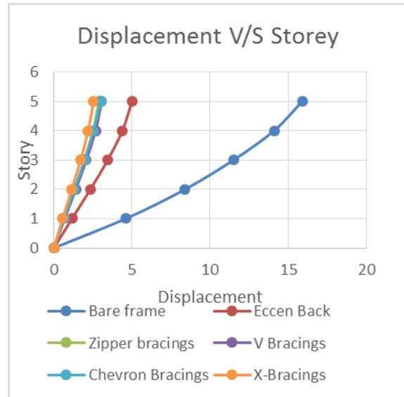
Fig. 2: Storey v/s Displacement Plot for 5 storey structure in x direction (zone-5)
