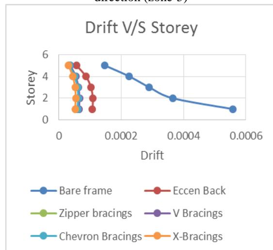
Fig. 7: Storey v/s Drift Plot for 5 storey structure in Y direction (zone-2)
