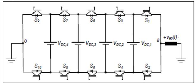
Fig. 8: Packed U-Cell (PUC) Topology
