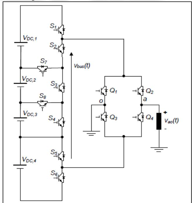
Fig. 10: Reversing Voltage (RV) Topology
