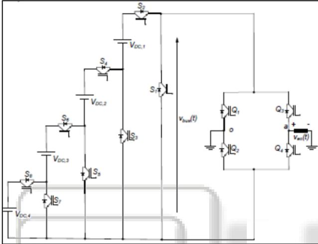
Fig. 6: Series Connected Switched Sources (SCSS) based MLI.
