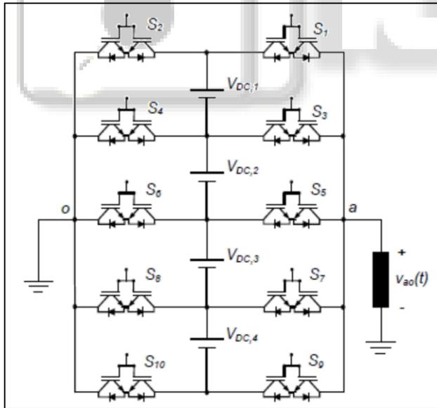
Fig. 7: Cascaded ‘Bipolar Switched Cells’ (CBSC) based MLI.
