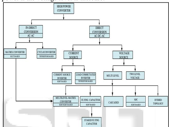
Fig. 1: Topologies of multilevel Inverters
