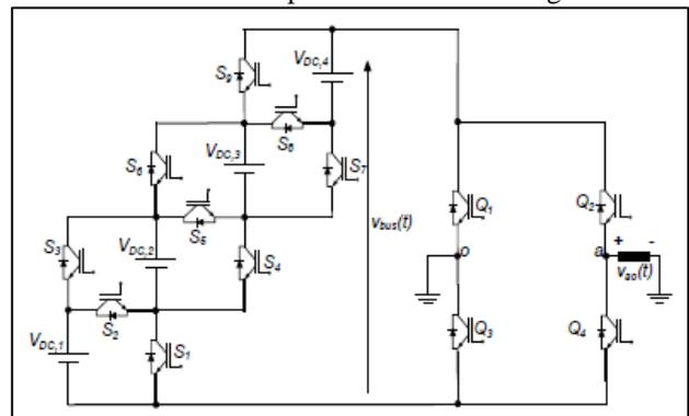
Fig. 5: Switched Series/Parallel Sources (SSPS) based MLI
