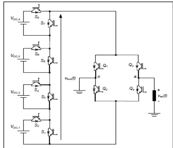
Fig. 3: Cascaded Half-Bridge based Multilevel DC Link (MLDCL)
