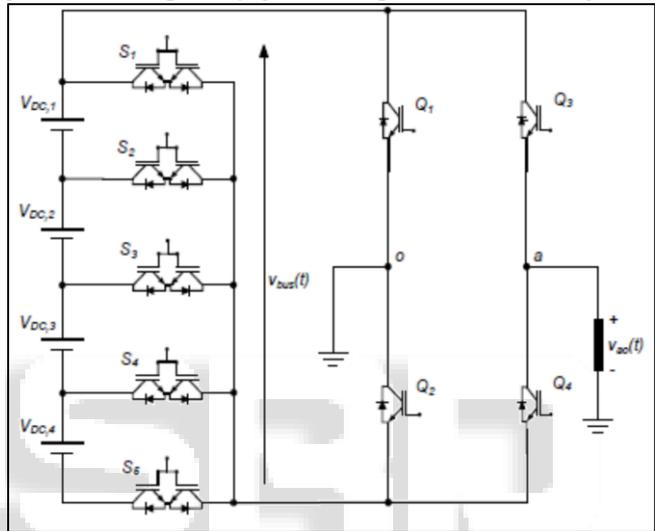
Fig. 9: Multilevel Module (MLM) based MLI
