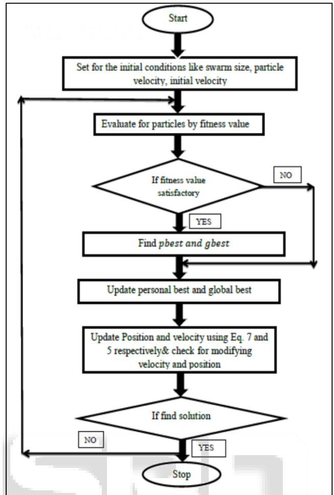
Fig. 2: Flowchart showing PSO algorithm
