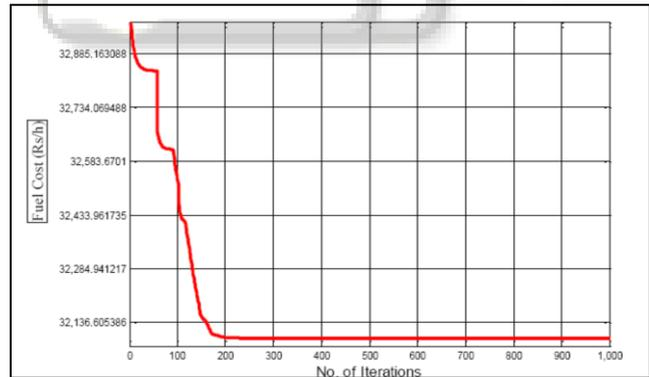
Fig. 4: Convergence characteristics with transmission loss for 600 MW
