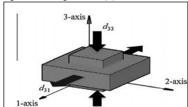
Fig. 1: operation modes and reference axis
