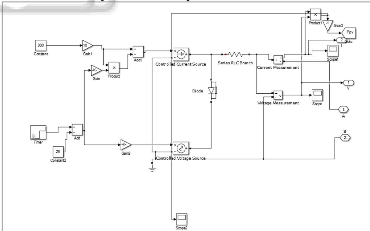
Fig. 3.2: Simulink Modelling of Solar system.
