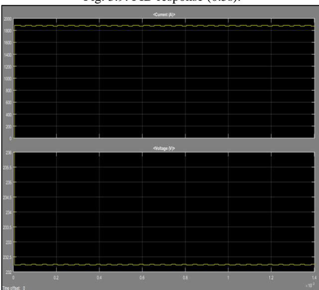
Fig. 3.10: Battery Storage voltage and current.
