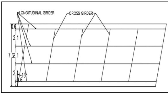
Fig. 3.3: Plan view of 15° skew integral bridge
