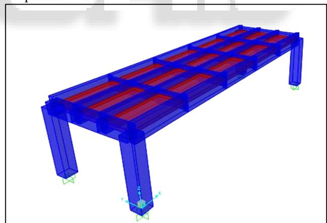
Fig. 3.1: Three-dimensional model skew integral bridge in SAP2000
