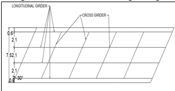
Fig. 3.4: Plan view of 30° skew integral bridge
