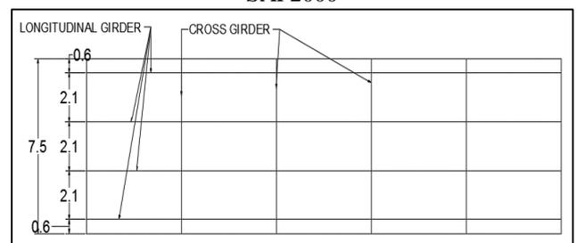
Fig. 3.2: Plan view of 0° skew integral bridge
