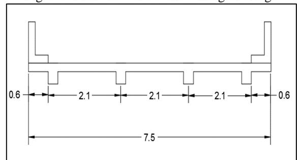
Fig. 3.7: Cross Sectional view of skew integral bridge
