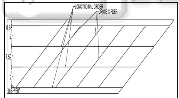
Fig. 3.6: Plan view of 60° skew integral bridge
