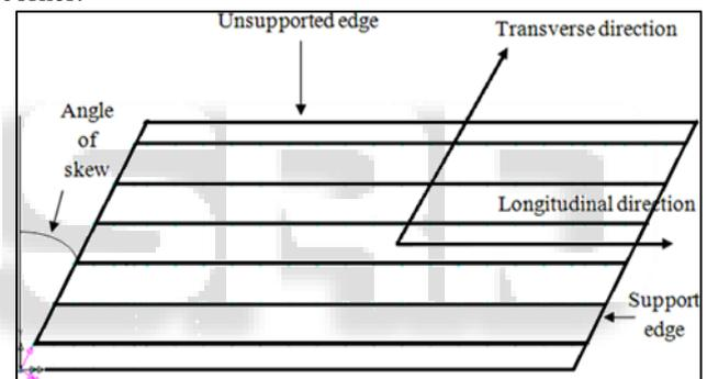
Fig. 1.1: plan of skew angle
