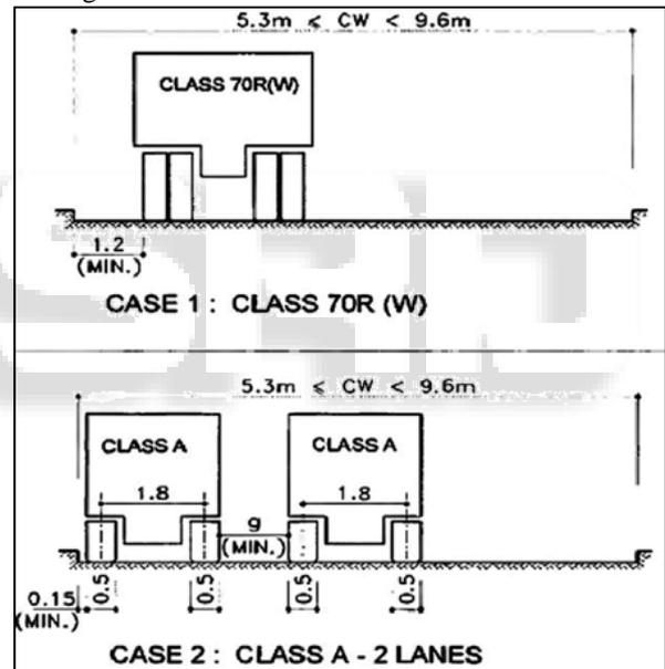
Fig. 3.8: Live Load combination as per IRC 6 2014 code
