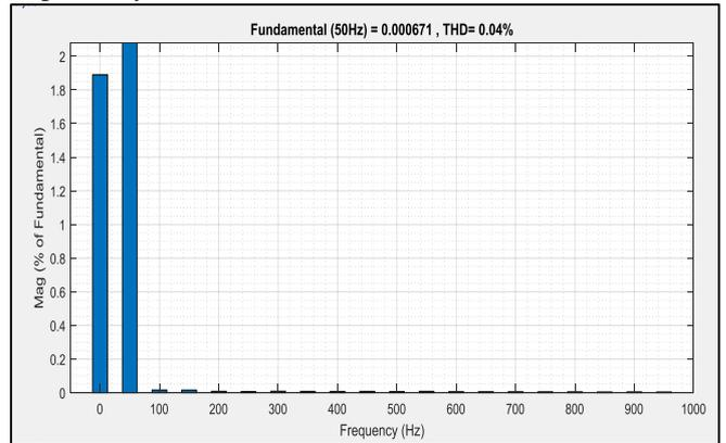
Fig. 7: FET analysis of load current where THD is 0.04 %
