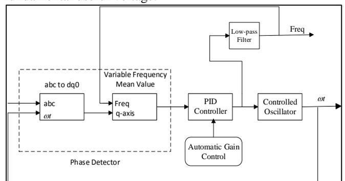
Fig. 4: Internal Diagram of PLL Controller
