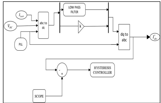
Fig. 3: Synchronous d-q-0 reference frame-based compensation algorithm
