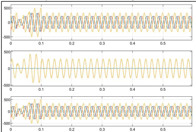
Fig. 6: (a) Three-phase Input Voltage (b) Compensating Voltage (c) Load Voltage
