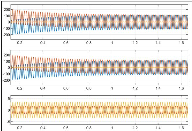
Fig. 5: (a) Source Current (b) Distorted Input Current (c) Improved Current
