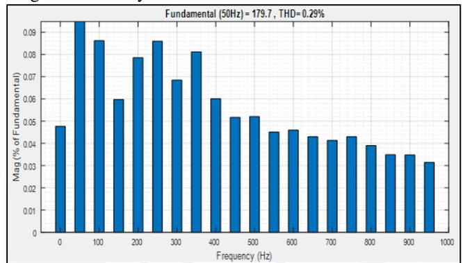
Fig. 8: FET analysis of load current where THD is 0.29%
