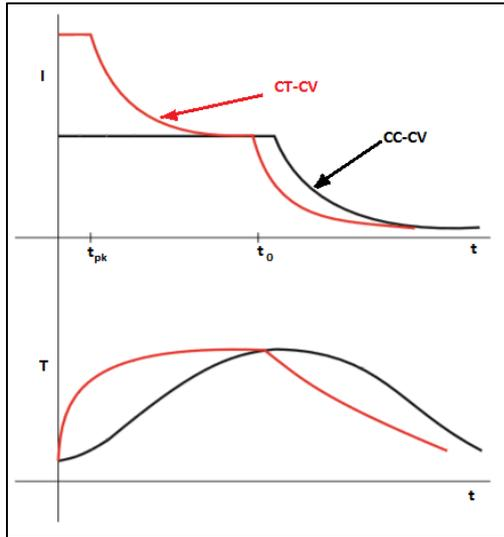
Fig. 2: CT-CV charging current and temperature variation with time
