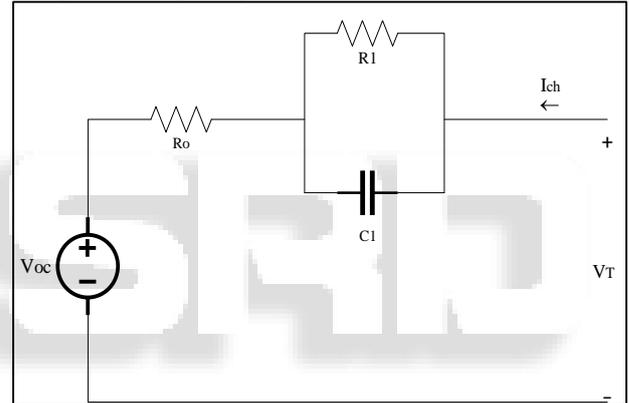
Fig. 3: Electrical model of battery
