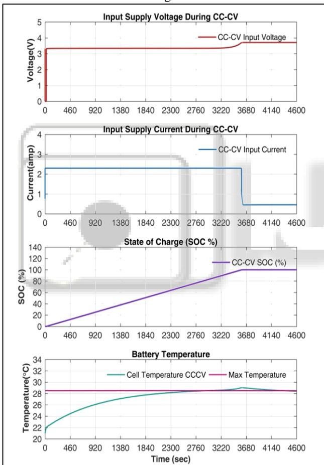
Fig. 5: Simulation results of CC-CV charging method for 3.7V lithium ion Battery at 0% SOC, Waveform of input supply voltage, input supply current, state of charge, battery temperature.
