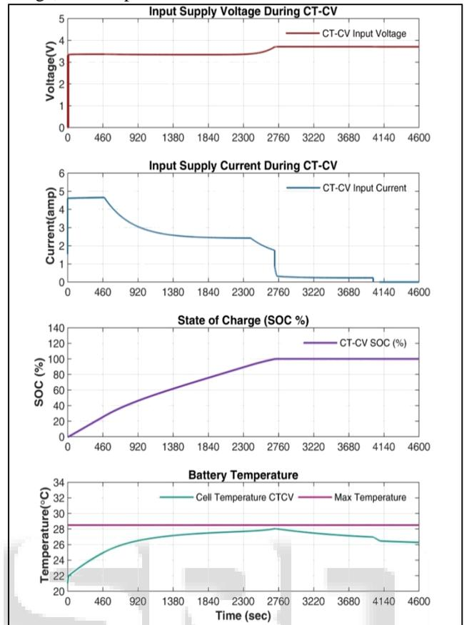
Fig. 6: Simulation results of CT-CV charging method for 3.7V lithium ion Battery at 0% SOC, Waveform of input supply voltage, input supply current, state of charge, battery temperature.
