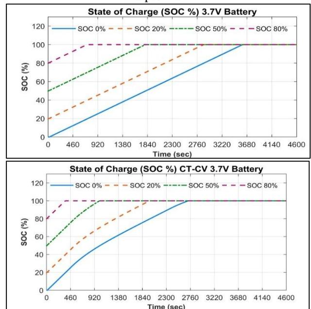
Fig. 7: Response of Battery SOC for 3.7 V Lithium-ion Battery for Both the Schemes
