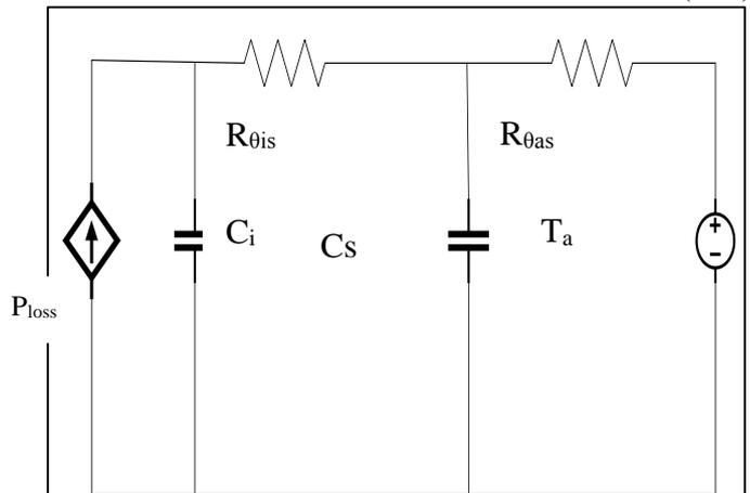
Fig. 4: Thermal model of Li-ion cell
